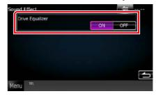
The sound quality is automatically optimized to meet the current volume level.
